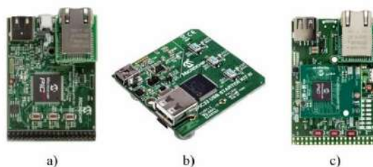
3-rasm. “Microelektronika”ning elektron platalari: a) PIC32MZ Connectivity EC Starter Kit; b) PIC32 USB Starter Kit III; c) Microchip PIC32MZ EF Starter Kit.
