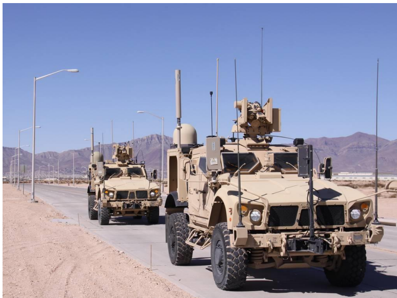
3-rasm. SNE (Soldier Network Extension) maxsus sun‘iy yo‘ldosh aloqa uskunalari bilan jihozlangan transport vositasi
